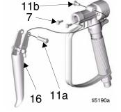
3. Before installing trigger, grease the actuator pins (7) and the pivot pin (11a).
