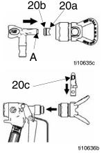
Install tip cylinder (20c) as shown. Turn 90° counterclockwise to spray position, so the arrow faces forward. Install assem
